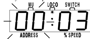
2. Press the
